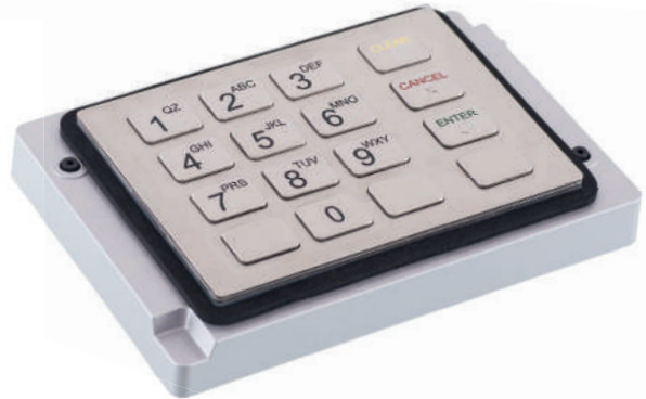
USB variant mounted in a 66xx compatible housing with USB interface board
