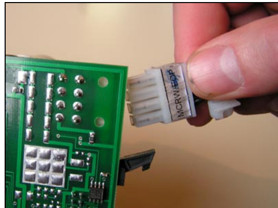
Connect power supply cable (5V, 24V and GND) to MCRK's MINIFIT 8M connector
